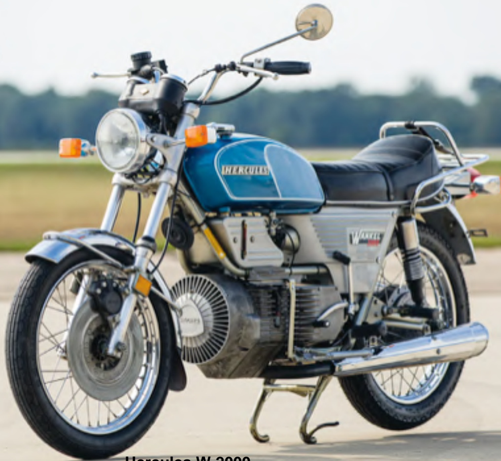
Hercules W-2000 the first production motorcycle with a Wankel engine.
