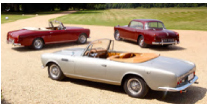
The Alvis Three Litre Series III sports saloon or drophead coupé, also known as TE 21 , was produced by English manufacturer Alvis between 1963 and 1966. The 3.0L engine, had power of 130 bhp (97 kW) at 4000 rpm giving the car a top speed of 107 mph (172 km/h).
