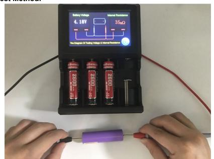
Access to the matching test pens, the red one is connected to the positive pole of the battery and the black one is connected to the negative pole of the battery. Hold and wait for 3 seconds, displays the actual voltage and internal resistance.
