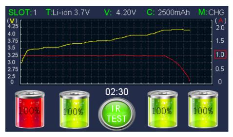
After putting multiple batteries, click the battery icon which one the users want to check; the battery icon turns red, and all the information at the top of the main interface is the information of the selected slot.
