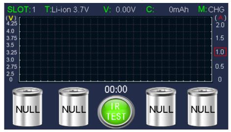
3) Access to the battery, if the users click the battery icon to enter the Settings Interface within 5 seconds, the charger will work as the setting parameters. Otherwise, it will automatically enter the default charging mode. As the following figure shows:
