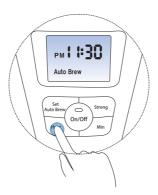
Step-3: Press On/Off button once, the light above On/Off button will light up in green colour, the Auto Brew indicator on the screen appears and the coffee maker directly enters Auto Brew mode.
