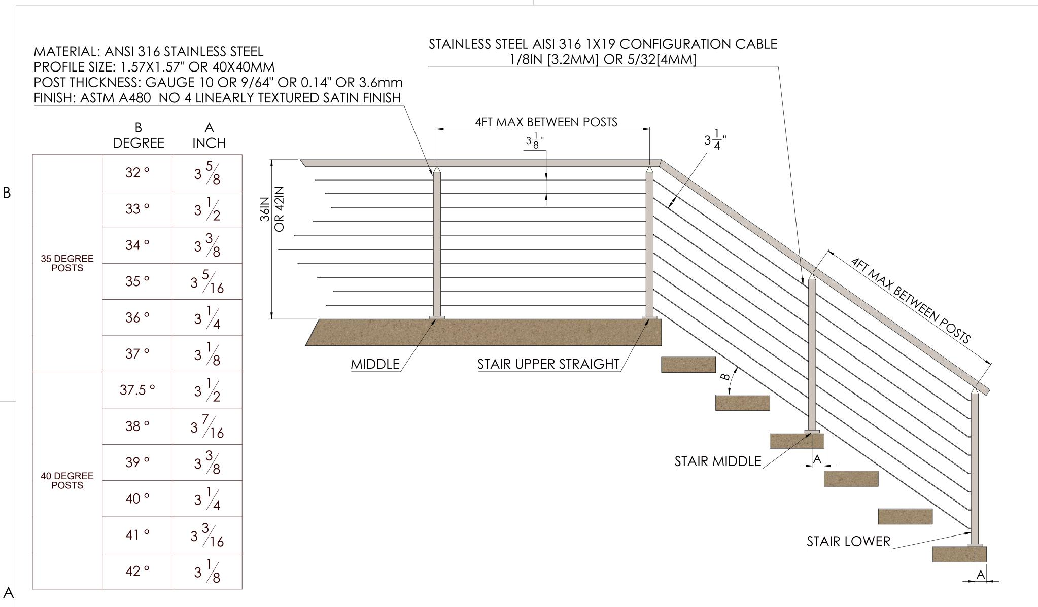
MEASUREMENT A: RECOMMENDED PLACEMENT DISTANCE FROM THE STAIR NOSE TO THE CENTER OF THE STAIR POST
