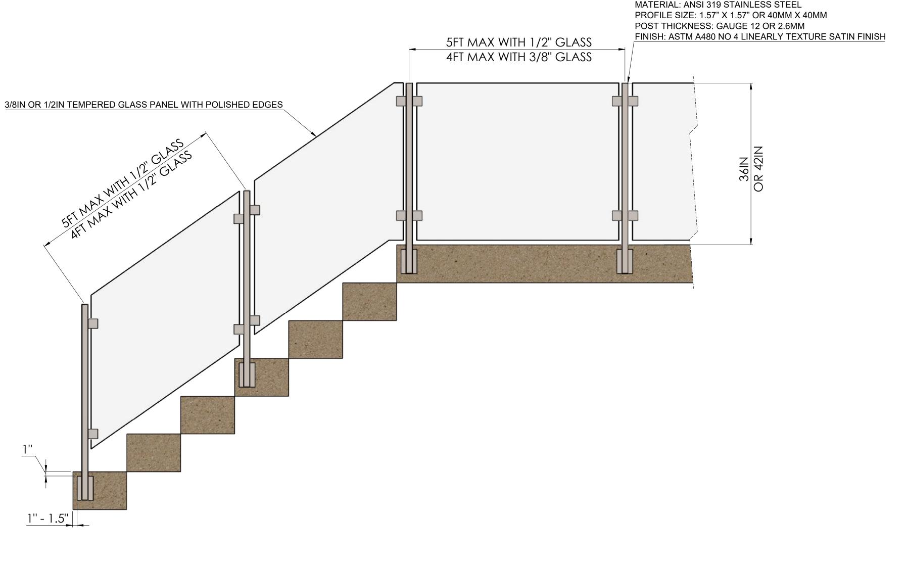
STAIR POST'S RECOMMENDED PLACEMENT: 1" FROM TREAD SURFACE TO TOP EDGE OF FASCIA PLATE & 1 - 1.5" FROM NOSE TO FRONT EDGE OF FASCIA PLATE
