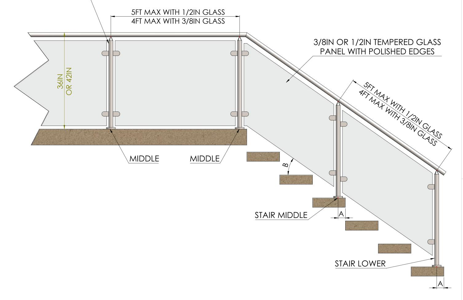
MEASUREMENT A: RECOMMENDED PLACEMENT DISTANCE FROM THE STAIR NOSE TO THE CENTER OF THE STAIR POST
