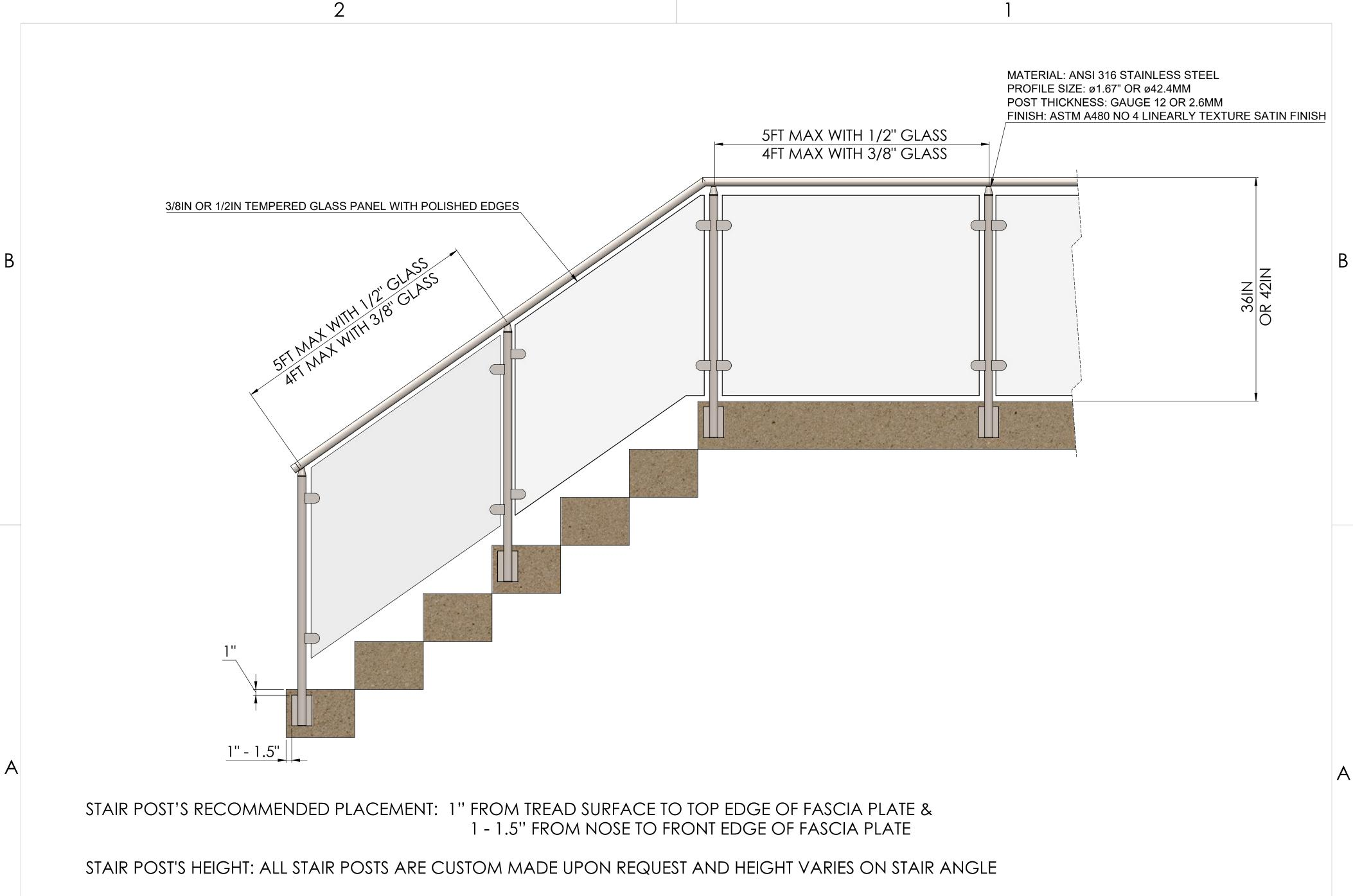
NOTE: THE USE OF THE SUPPLIED GLASS CLAMP PIN IS REQUIRED TO SUPPORT LARGE GLASS PANELS
