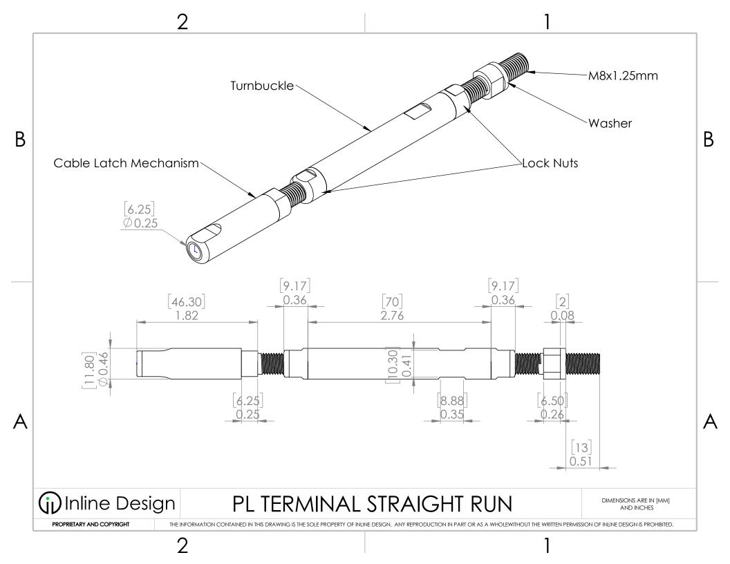
В [6.25] Ø 0.25 M8x1.25mm Washer [13] |0.51 9.80 [46.30] 1.82 (i) Inline Design PL TERMINAL STRAIGHT RUN DIMENSIONS ARE IN [MM] AND INCHES PROPRIETARY AND COPYRIGHT
