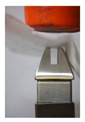
*NOTE:* If the bracket doesn't align properly you can tap it out using a 1" rod from the bottom of the post. Be careful not to hit any of the tube threading while inserting the rod. Do this over a piece of cloth so that they bracket does not get scratched when it is tapped out.
