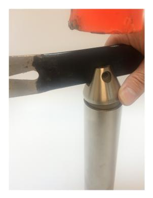
*NOTE:* If the bracket doesn't align properly you can tap it out using a 1" rod from the bottom of the post. Be careful not to hit any of the tube threading while inserting the rod. Do this over a piece of cloth so that they bracket does not get scratched when it is tapped out.
