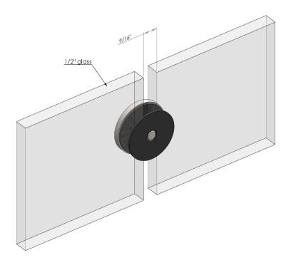
Step 3: Loosely screw the other plate through the threaded rod by hand and insert the Allen wrench through the slot to finish tightening the plate
