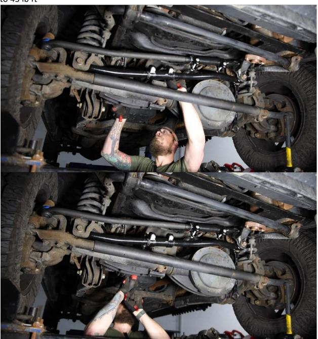
8. We recommend that you double check all work and add paint marker lines to all torqued bolts so you can monitor any possible loosening of components.
