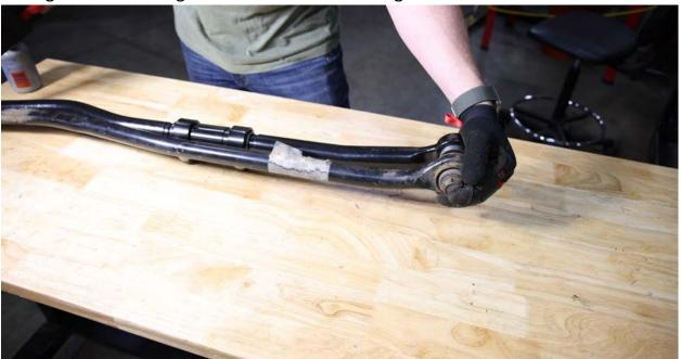
4. You can now put the YETI XD™ track bar back in the vehicle, starting with the passenger side mount and putting the track bar bolt in there first, and then putting the driver's side end into the mounting location and putting the track bar bolt in to hold it in position. If you have adjusted the track bar properly in the previous step then your axle should remain centered.
