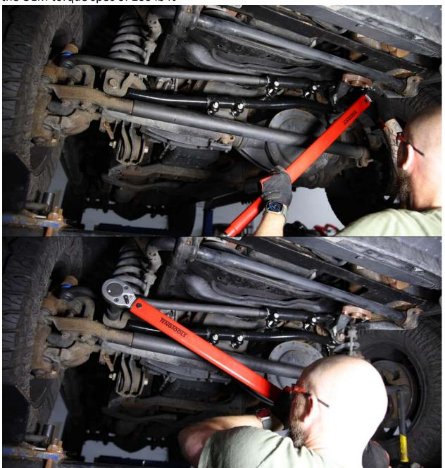
6. If you've installed a lift with the track bar, now would be a good time to go ahead and center the axle. Measuring from a consistent static point on the frame to a consistent static point on the tires, turn the adjuster sleeve on the track bar to shorten or lengthen the track bar until the axle is centered underneath the vehicle.
