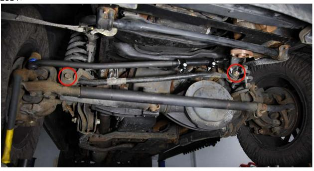
2. Assemble YETI XD™ Front Adjustable Track Bar – we recommend that you use anti-seize on the threads. Threads are right-hand and left-hand and will only thread into one side of the adjuster sleeve.
