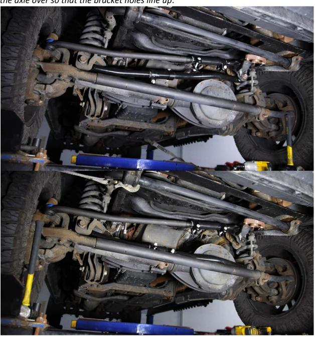
5. Making sure the vehicle is sitting at ride height with the weight of the vehicle on the axle, you can now torque the track bar bolts back down using the OEM torque spec of 200 lb ft
