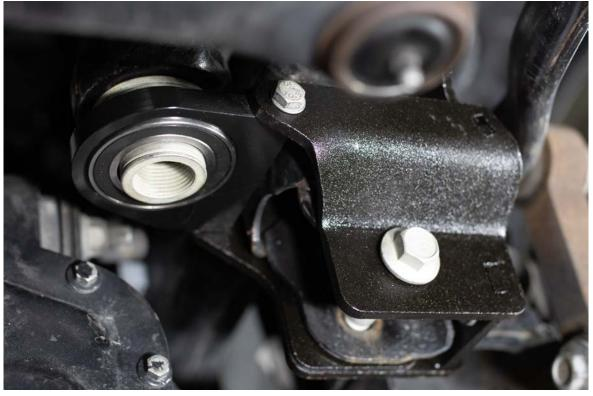
13. Install the c-clip beneath the roller bearing plate in the sector nut channel
