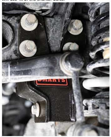
Use the 19mm socket and torque to the following spec (for the steel box you can reinstall plug after torqueing): 2x Long Bolts (aluminum box): 44 ft lbs + 170°
