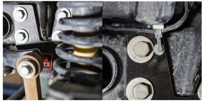
9. Now install the Steer Smarts sector shaft nut. Place **1x** washer on the sector shaft above the sector shaft nut and then thread the sector shaft nut onto the sector shaft. We recommend applying some Red Locktite at this point. (there are 2x washers included in the kit – use both washers if your specific application requires it for proper spacing/tolerance to snap ring)
