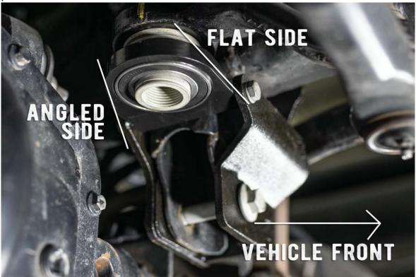
For any issues with the bearing plate not lining up with bolt holes, you may need to loosen the steering box bolts to adjust the plate for everything to align properly – the holes for the steering box and the track bar mount are slightly oblong and can be adjusted slightly for proper alignment.
