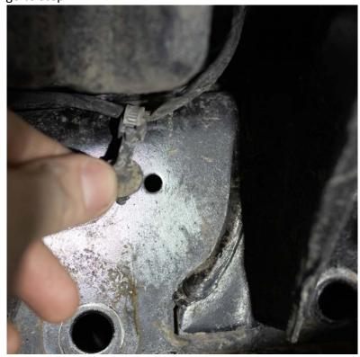
Measure approximately 1" to the right from the center of the top hole on the left side of the bracket. Using a center punch tool (or marker).
