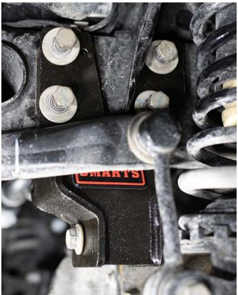
Use the 19mm socket and torque to the following spec (for the steel box you can reinstall plug after torqueing): 2x Long Bolts (aluminum box): 44 ft lbs + 170° 2x Short Bolts (aluminum box): 44 ft lbs + 135° 4x short bolts (steel box): 44 ft lbs + 135°
