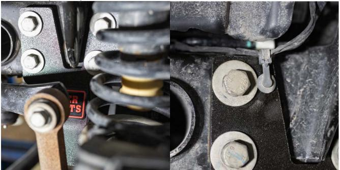
9. Now install the Steer Smarts sector shaft nut. Included are two washers that are used as spacers. Place the two washers on the sector shaft above the sector shaft nut and then thread the sector shaft nut onto the sector shaft. We recommend applying some Red Locktite at this point, too.
