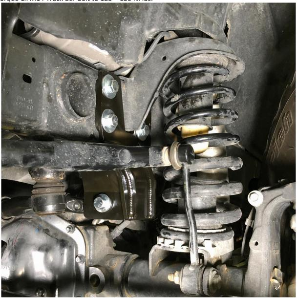
7. You have successfully installed the Frame Side Track Bar Reinforcement Bracket
