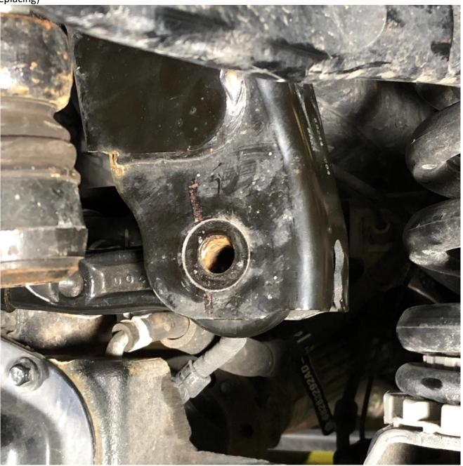
2. Using 18mm - remove 4x fasteners holding Power Steering Gear Box:
