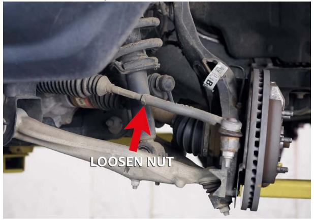
3. Remove tie rod nut. Use a hammer to tap on bottom of stud to unseat from knuckle. Unthread outer tie rod end and then unthread and remove jam nut.
