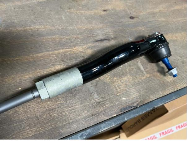
6. Measure the length from line to center of Yeti XD Outer stud and then place Outer stud through the factory mounting position and torque nut to 46 lb ft.
