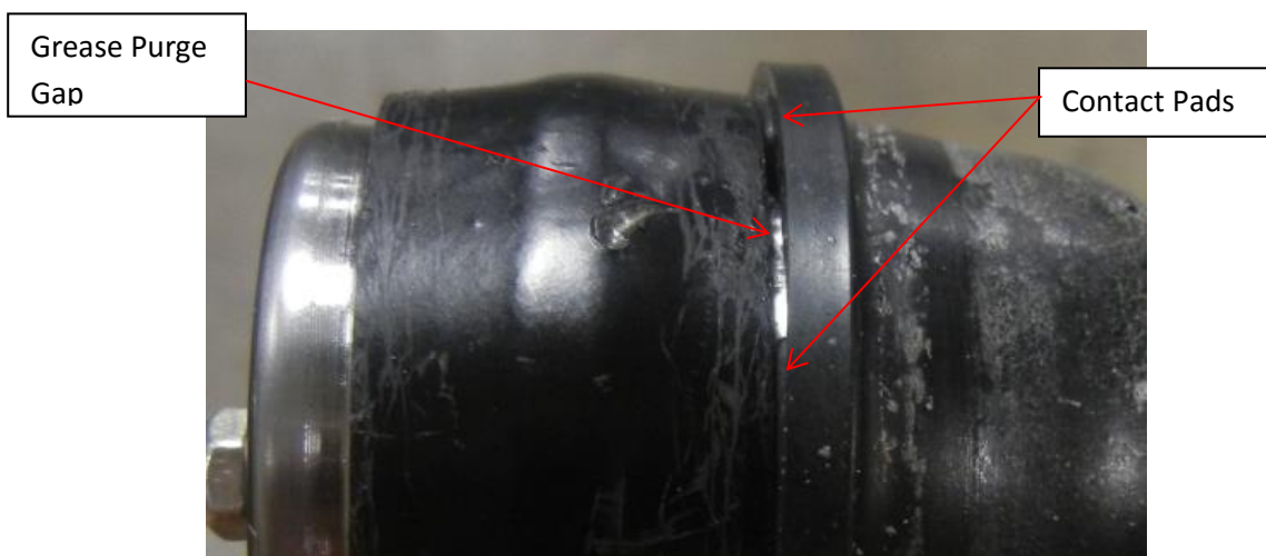
Figure 8: Properly Installed Seal Height
