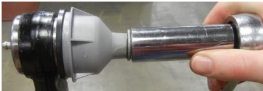
Figure 11: Torque Seal in Place
