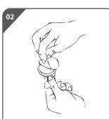
Before turning the device ON remove and discard the *Electrode Gel Pad Sticker* ( ). Stick one gel pad onto each electrode of TANYX device. This Electrode Gel Pad will remain until
