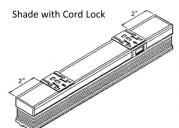
Position the first two installation brackets so that they are approximately 2" in from the end of the headrail. If a third bracket is included, center it between the outer brackets. Wide shades may include up to 8 brackets. In these cases, space the additional brackets evenly, not more than 25" apart. Mark the brackets for mounting hole locations, making sure they are square and equally spaced. For outside mount installations, use a level to check for levelness.
