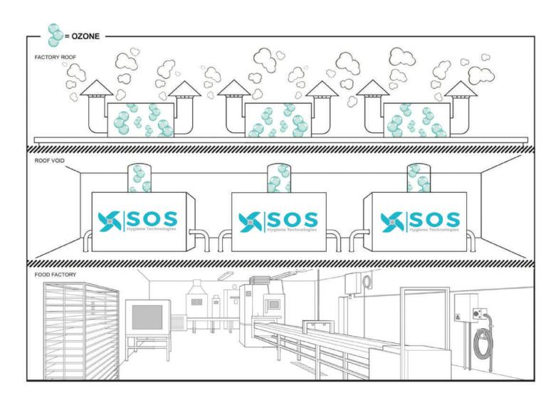
Common compounds that have been identified in industrial odours (sulphides, amines and mercaptans) are effectively neutralised. Despite claims, ozone cannot oxidise ammonia, however it can eradicate all ammonia-producing microorganisms and therefore can reduce ammonia formation.
