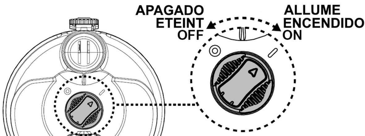
Turn the power switch on and off as shown in the diagram above..
