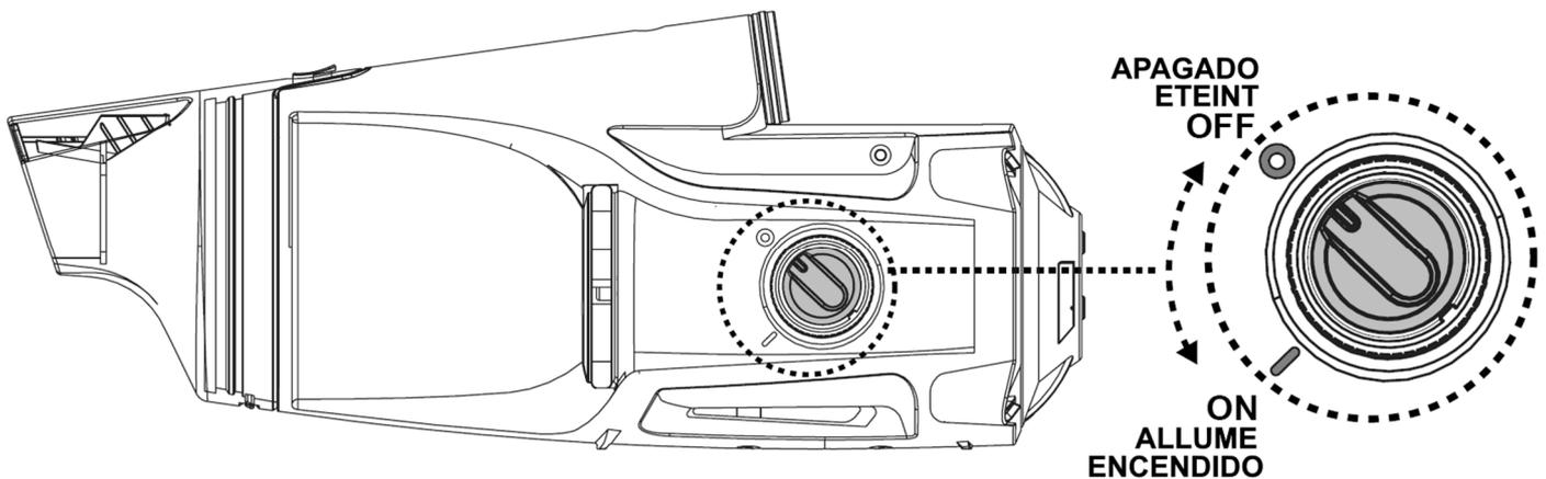
Turn the power switch on and off as shown in the diagram above..
