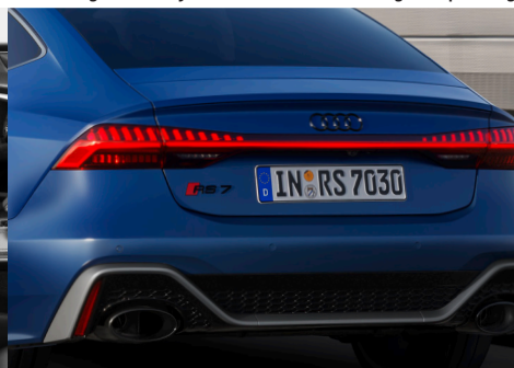
LED rear lights with dynamic indicators and RS light sequencing
