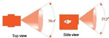
Scan angle in non-repetitive mode
