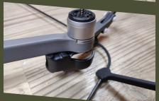
Step Four: Connect the back legs of the drone by firmly pressing the leg into the rear connectors.
