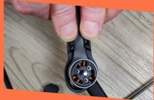
Step Two: Remove the front connector by firmly pushing the sides of the connectors around the drone's arms with your thumbs. You can now remove the drone from the cage.
