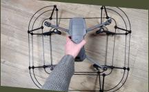
Step Two: Place the drone into the cage through the top aperture.
