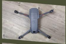
Step One: Unfold your Mavic 2 series drone and remove any connected propellers. Place the cage on a flat surface.
