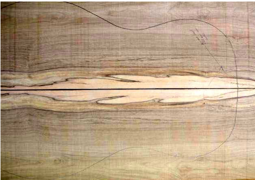
Figure 22 Native olive or dorrall ( Notelaea ligustrina ) acoustic guitar back under construction
