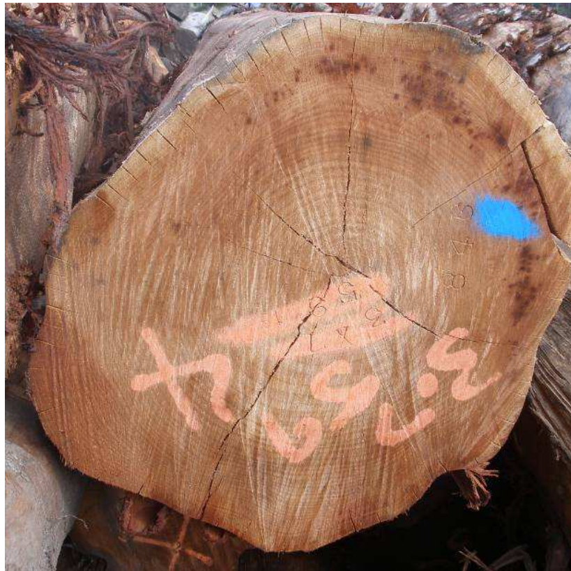
Figure 4. Silver wattle log; 59cm large end diameter of approximately 48 years from southern Tasmania. (Phillips Sawmill, Geeveston 2007)
