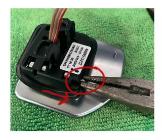
Once the pin is pushed out enough it can be grabbed with the small needle nose pliers and be pulled out of the paddle assembly fully.
