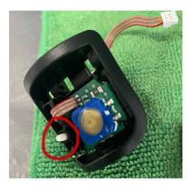
Make sure the small white piece of plastic does not fall out of the electronic section of the paddle, as it is what helps the shift paddle be tight in its assembly
