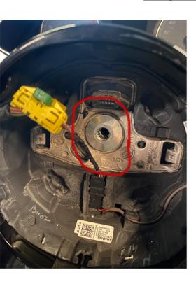
Using the 12mm triple square, remove the center bolt from the steering wheel.
