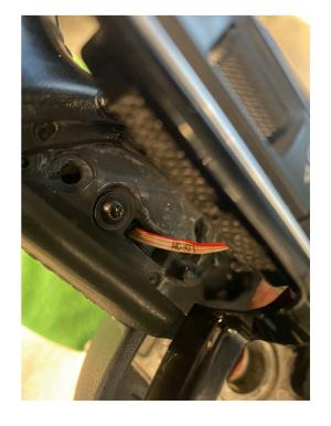
Once the trim is separated, there is wiring from each shift paddle to the steering wheel controls, disconnect these wires from the back of the steering wheel controls.
