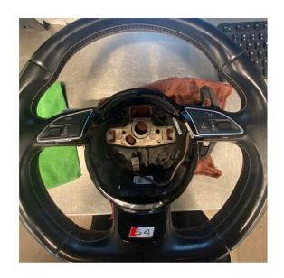
Using the plastic pry tool, insert and pry between the steering wheel leather and the plastic trim that surrounds the airbag and steering wheel controls.
