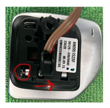
Pictured right, the holding pin is being pushed out of the top
