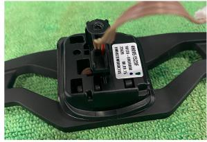
Insert the pin into the assembly to hold everything together, this should fit exactly like the OEM paddle.
