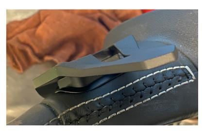
Once the new paddle is installed onto the electronic section, reinstall the assembly into the steering wheel.
