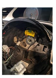
Pictured above is the airbagclip that needs to be released.
