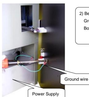
Be sure to connect the connectors firmly.Ground wire has to be connected the Main Body with Screw.
