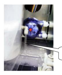
10) Set a Drainage Pipe to 2nd Tank.
