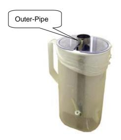
2) Set an Outer-Pipe with the Reactive Pipe inside the cover.
