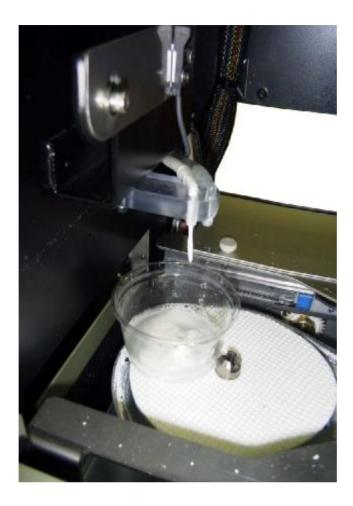
Turn on a compound pump and a water pump until a compound and water appear from nozzles.
