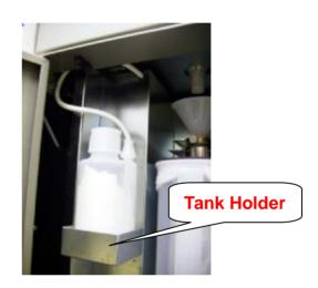
11) Pour over 200 ml of Compound into Compound Tank and set it in Tank Holder.
