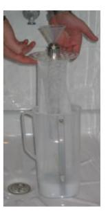
3) Pull out the Reactive-pipe from Outer-Pipe by loosing the small screw.
