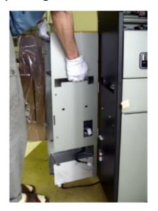
1) Insert each Hinge on Changer into both of Hinges on the Main Body referring to the picture, respectively.
