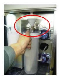
11) Drainage Pipe has to be turned and put into the hole of 2nd Tank.
