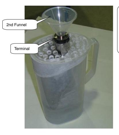
3) A terminal is fixed to the Inner-Pipe with a terminal fixed screw.
