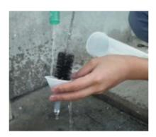
7) Put 1st Filter in 1st Tank and turn the end outside. Expand inside of the 1st Filter.
