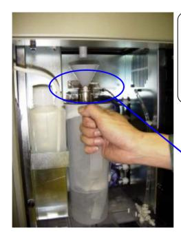
9) Set a 1st Tank on 2nd Tank.Make sure that Terminals has to be connected firmly.
