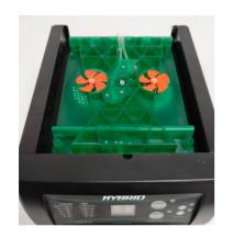
With the lid in the open position you need to remove the 4 screws in the recess of the green inner lid which allows you to take off the black top cover. Use the smaller screwdriver for this.
