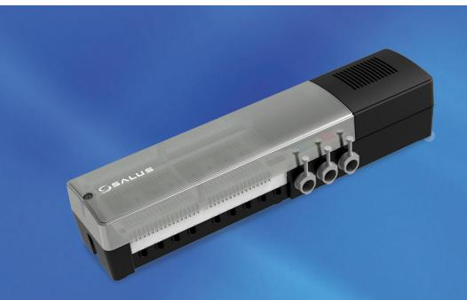
The SALUS AKL08RF Relay Controller for underfloor heating systems is the perfect interface between thermostats and actuators. It ensures precise control for optimum comfort and efficiency. Volt-free connections for Pump and Boiler integration, 120 VAC power input, 24 VAC outputs, and Night Set Back control allow the AKL08 to fit any situation.
