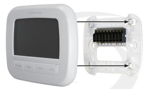
Attach Display to Mounting Plate: Line up sockets in the back of the thermostat with the posts on the wall plate and snap it into place. Make sure the connector pins are not bent and wires do not interfere with the thermostat engagement. The thermostat must be fully seated on the wall plate to operate correctly.
