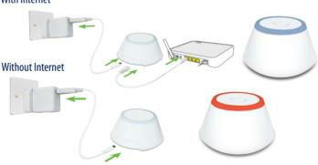
If you are installing an underfloor system without an Internet connection, you can use the coordinator from the AKLO8RF instead of the Universal Gateway.
