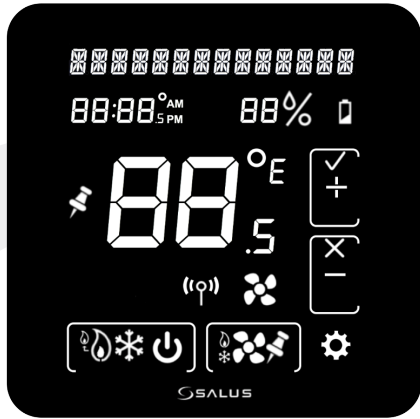
3 second display of all LCD segments
