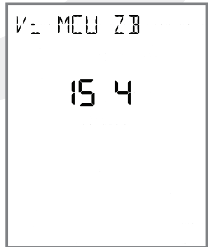
Displays MCU and Zigbee firmware version for 3 seconds
