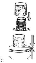
Carefully slide the foam wet filter down over the filter cage making sure the cage is completely covered.
