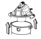
Lift the power head off the collection tank.
