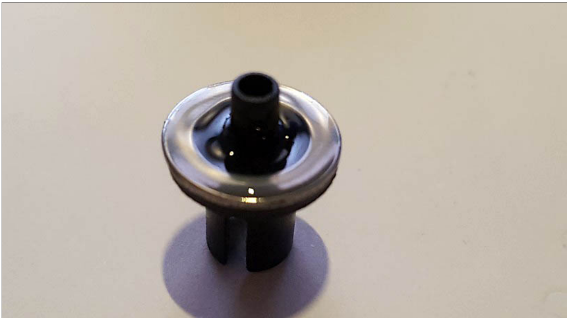
Step 3: Place a 3x6x2mm ball bearing into diff gear and place onto above cup assembly:
