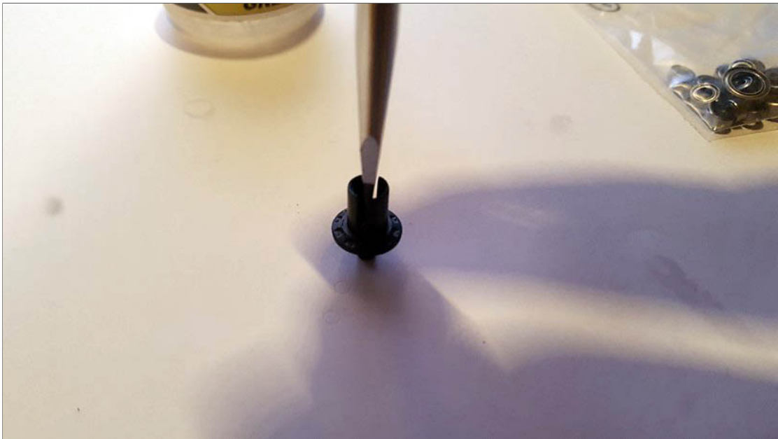
Step 2: Place a pressure plate onto the cup and apply Ball Diff Grease
