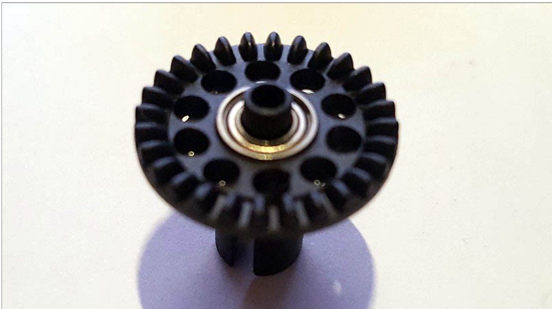
Step 4: Apply Ball diff grease and place 10x 2mm steel balls into the gear, don't drop them!
