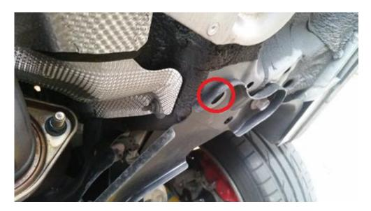
**2.8.** We can now install the front panel. First bolt the 17mm bolt with the panel now on top of it. Tighten this to 48 ft-lbs.
