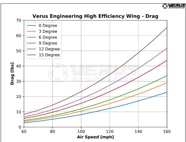
Freestream downforce data on the Verus Engineering High Efficiency Wing which is on the Ventus 2 Package. The data on the car on the previous page is from 6 degrees angle of attack. How the downforce and drag can change based on wing angle change can be calculated using these graphs.
