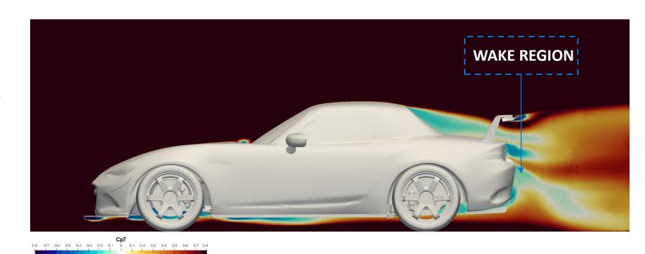
The CpT Plot shown above is used to visualize the wake region behind the car. The blue zone behind the vehicle is the wake and minimizing this as much as possible will reduce drag.
