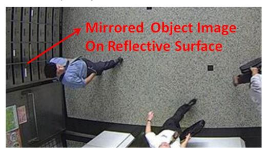
9. If the human detection is applied, the shooting angles of the FD9369, IB9369 and box camera with non i-CS lens should be 60° or above to acquire better analysis results.
