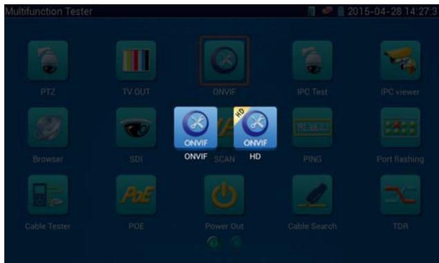
If you select ONVIF SD or HD mode, the tester automatically scans different network segments for ONVIF cameras. It lists the camera name and IP address on the Device List. If no cameras appear under the device list, try clicking on the Refresh button
