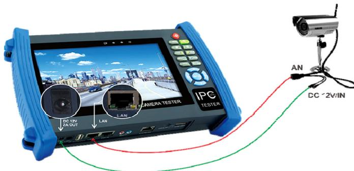
Note: If the link indicator of the tester's LAN port is green and the data indicator flickers, it means the IP camera and the tester are communicating. The tester's upper right corner will show the icon.
