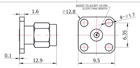
For glass-bead of 0.38mm pin diameter
