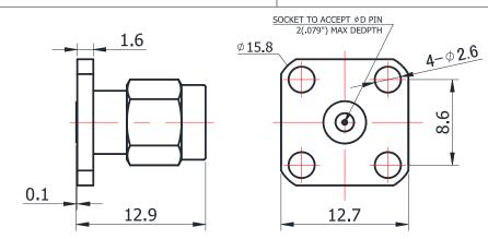
For glass-bead of 0.51mm pin diameter
