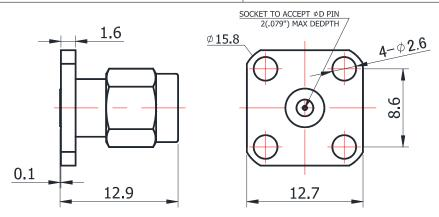
For glass-bead of 0.38mm pin diameter
