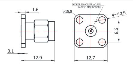
For glass-bead of 0.23mm pin diameter
