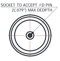
For glass-bead of 0.30mm pin diameter
