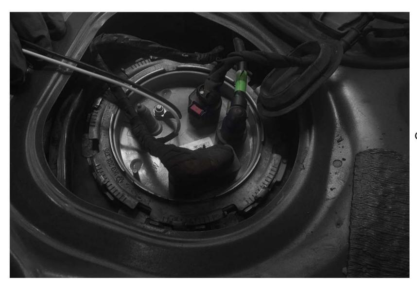
Connect the plugs and pipe back with fuel pump
