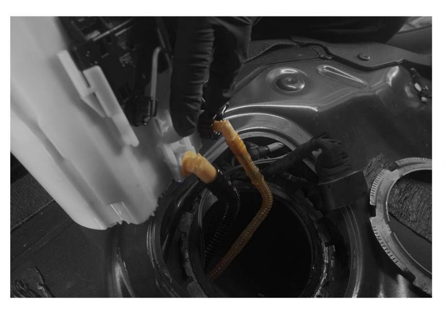
Take the fuel pump out and remove the two hoses
