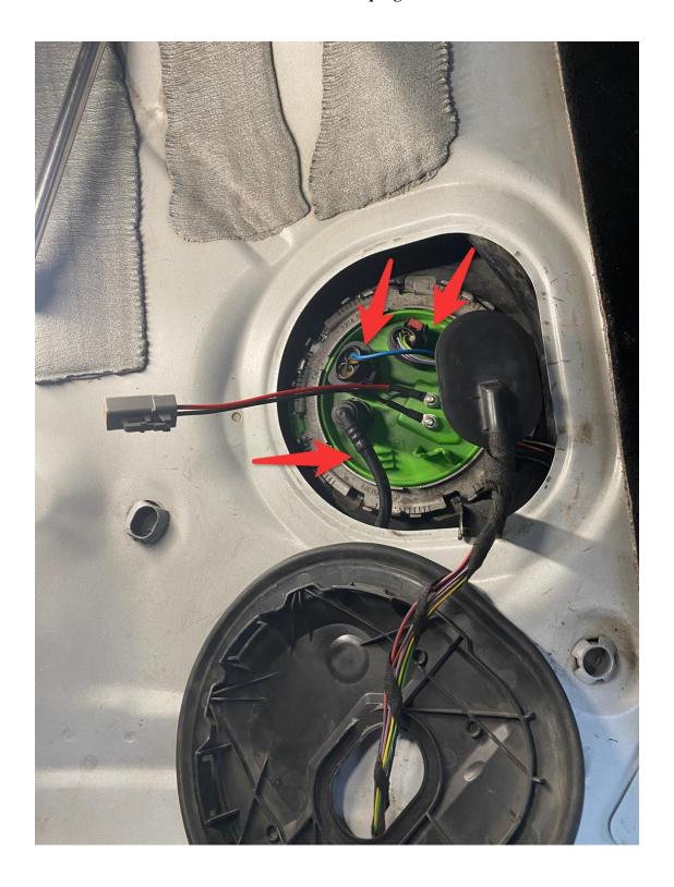
6. Auxiliary Plug Coming from relay and its must be connected with lpfp Auxiliary Plug.[Auxiliary Plug connected with relay]
