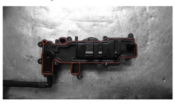
7.Install the OEM sealing washer onto the JDY PCV Valve
