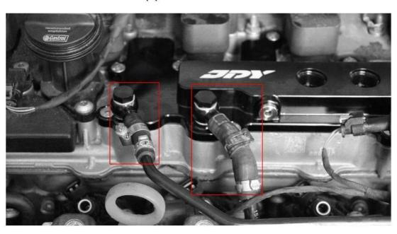
10.Install the JDY EGR(Exhaust Gas Recirculation) pipe fitting to intake pipe
