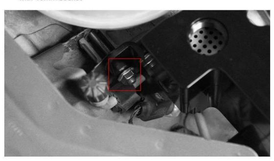
15.Fasten the bolt supplied from JDY on the JDY Oil Catch Can with H5 socket
