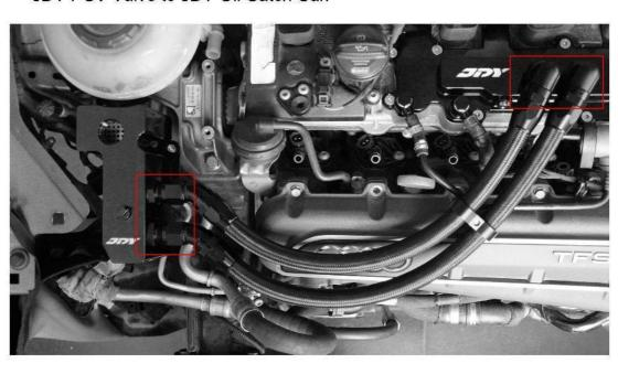
17.Connect the AN12 EGR(Exhaust Gas Recirculation) hose between the fitting on intake pipe and JDY Oil Catch Can
