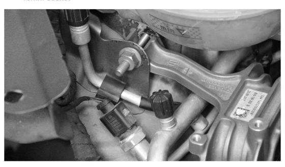
14.Fasten the screw nut supplied from JDY on the JDY Oil Catch Can with 13mm socket
