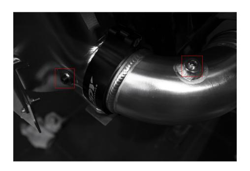
12.Install the clamp to secure the JDY scilicone charge pipe with 7mm socket
