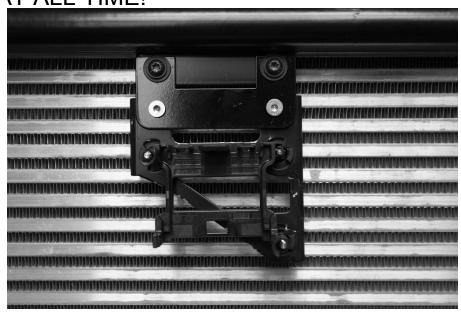
14: Install the JDY hook lock with T30 and H5 sockets
