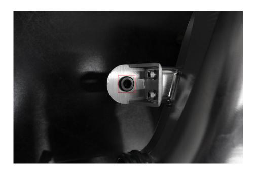
5 Install the JDY intercooler on the radiator support frame by fastening the bolts provided by JDY with H5 socket
