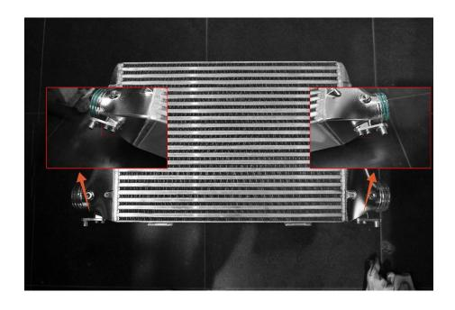
2.Install the upper intercooler bracket by fastening the JDY bolts with H5 socket
